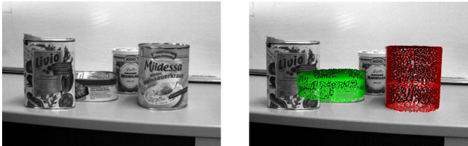
Fig. 4. Recognition result: 3D dot clouds projected onto left camera image
