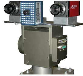
Fig. 3. Sensor head: Stereo cameras and 3D-TOF camera mounted on a pan/tilt unit
