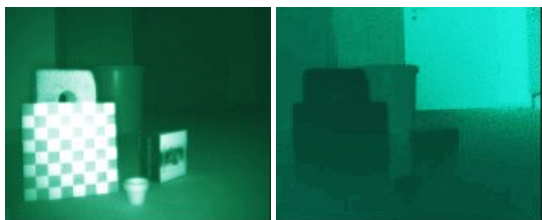
Fig. 2. Intensity (left) and depth (right) images of a scene containing a chess board and some little objects. The grey values mean different luminance in the intensity image and different distances in the depth image. Both are acquired by the same chip, such that we have exact and known pixel correspondences.
