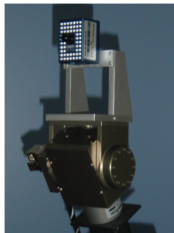
Fig. 3. The 2-DOF pan-tilt unit, a PowerCube PW70, with the mounted TOF-sensor. The available degrees are pan and tilt with the corresponding angles \phi and \theta .
